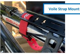
2. If you're attaching the light to a delicate surface you might want to add a protective tape of pad to keep the bracket from scratching any surfaces. The voile straps will provide a protective space between the light and the mount surface and this should suffice for protection.
